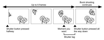
To eliminate the lag between the shutter button being pressed all the way down and the start of recording, the camera starts shooting a series of pictures using the electronic shutter when the shutter button is pressed halfway, and begins recording the pictures including those taken when the shutter button was pressed halfway (up to 5)—to the card when the shutter button is pressed all the way down.
